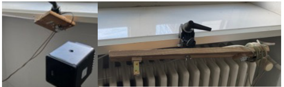
Figure 1: String mounting plates with guitar tuning peg and clamp; left: Piezo-side small plate with speaker cable and associated loudspeaker; right: Magnet-side longer board.
