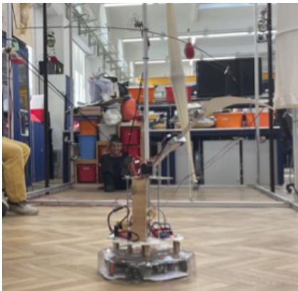
Figure 1: Claw, the robot used as avatar in the experiments of the first prototype.
